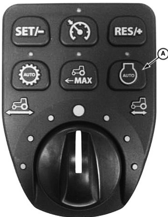
A—Interruptor del eThrottle
