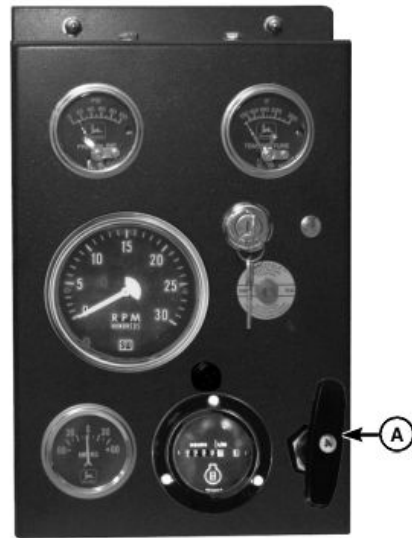
Throttle Handle on North American Instrument Panel
