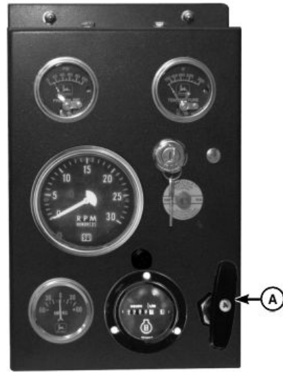
Throttle Handle on North American Instrument Panel
