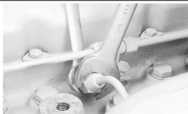
Bleeding Fuel System at Injection Nozzle
