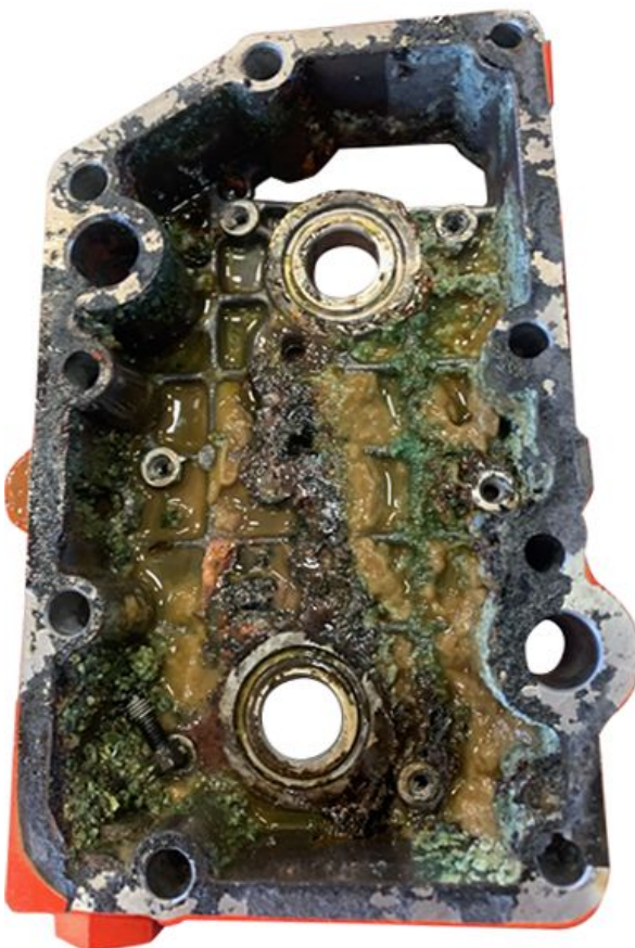
Effects of Prolong Storage of Coolant — More Than One Year
