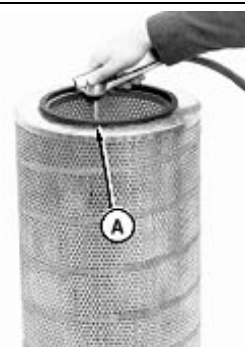
Cleaning Primary Element
