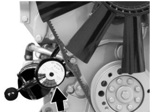
Checking Belt Tension with Tension Gauge
