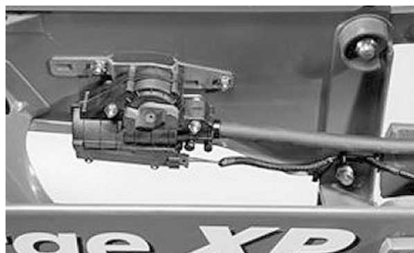
Embrayage RowCommand™ MaxEmerge™ Pro-Shaft
