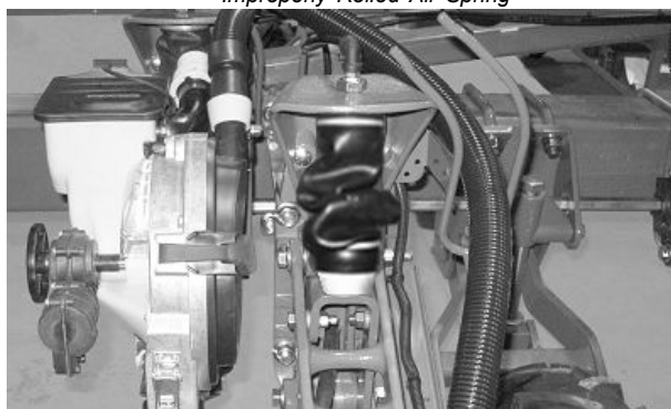
Improperly Rolled Air Spring (Twin Row)
