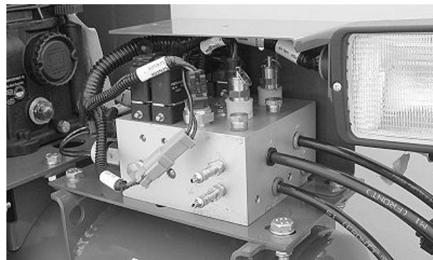
Pneumatic Down Force Pressure Sensors (Active Down Force) (Dual Set-Point Valve Shown)
