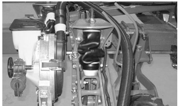
Improperly Rolled Air Spring (Twin Row Planters)
