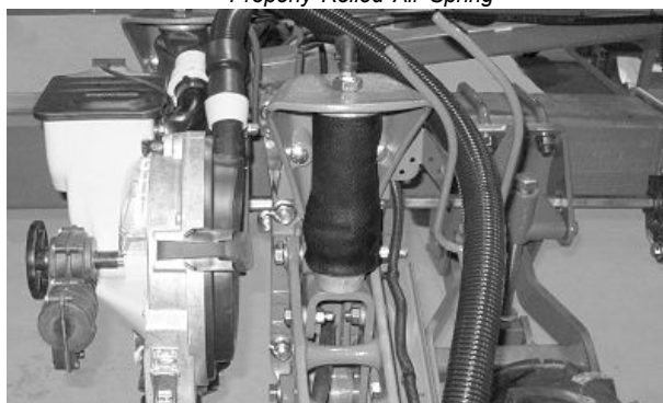
Properly Rolled Air Spring (Twin Row)
