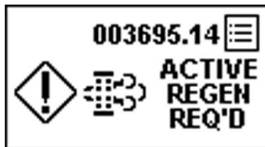
PY44599—UN—08SEP17 Auto Cleaning Required, Regeneration Disabled
