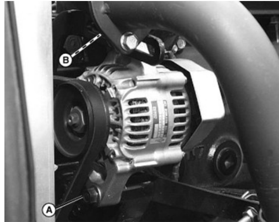
Alternator located on right side of engine.
