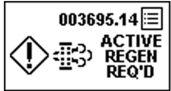
PY44599—UN—08SEP17 Auto Cleaning Required, Regeneration Disabled
