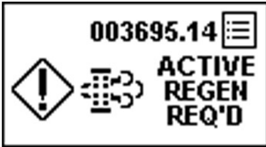
PY44599—UN—08SEP17 Auto Cleaning Required, Regeneration Disabled
