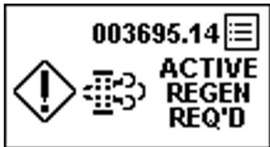
PY44599—UN—08SEP17 Auto Cleaning Required, Regeneration Disabled
