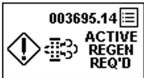
PY44599—UN—08SEP17 Auto Cleaning Required, Regeneration Disabled
