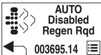
TCT012084—UN—26NOV14 Auto Cleaning Required, Regeneration Disabled
