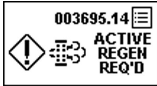
PY44599—UN—08SEP17 Auto Cleaning Required, Regeneration Disabled
