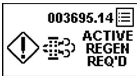
PY44599—UN—08SEP17 Auto Cleaning Required, Regeneration Disabled
