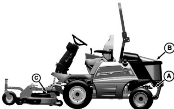
Clean out areas
