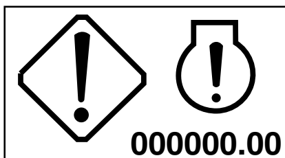
PY46275—UN—07SEP17 Generic Engine Fault - Warn Lamp Status
