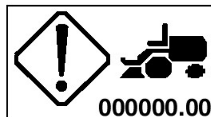
TC101636—UN—29OCT20 Generic Machine Fault – Warn Lamp Status
