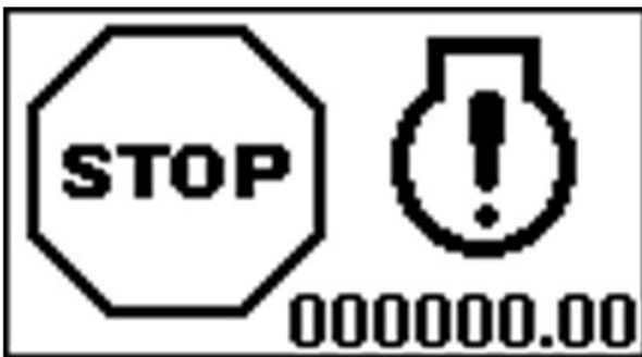
PY44596—UN—06SEP17 Generic Engine Fault - Stop Lamp Status
