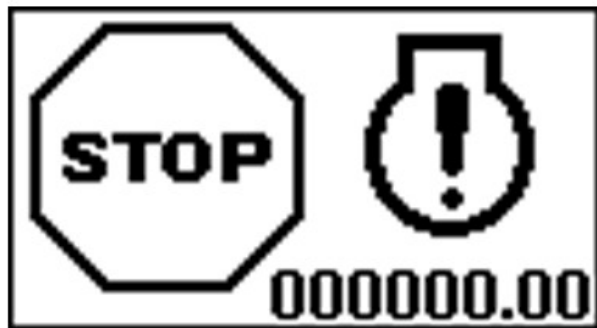
PY44596—UN—06SEP17 Generic Engine Fault - Stop Lamp Status
