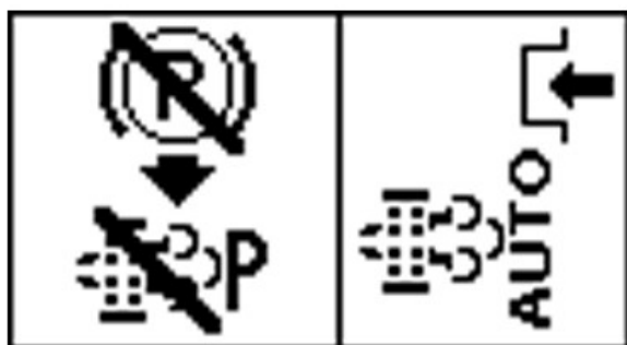
PY44594—UN—06SEP17 驻车制动器关闭，驻车再生互锁
