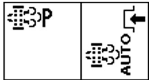
Parked Cleaning Required (Amber Warning Lamp)
