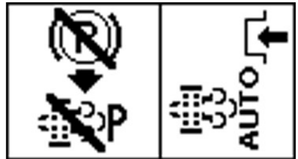
PY44594—UN—06SEP17 Park Brake Off, Parked Regeneration Interlock
