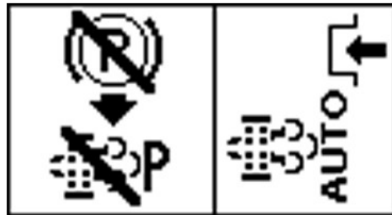
PY44594—UN—06SEP17 Park Brake Off, Parked Regeneration Interlock
