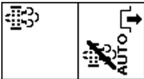
PY44610—UN—12SEP17 Cleaning Required - Auto Regeneration Disabled
