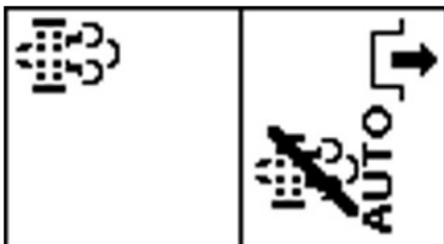
PY44610—UN—12SEP17 Cleaning Required - Auto Regeneration Disabled
