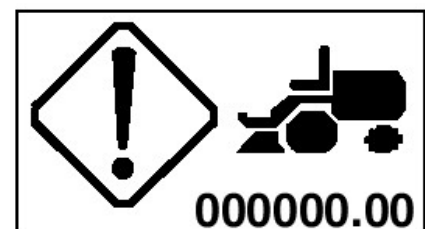
TC101636—UN—29OCT20 Generic Machine Fault – Warn Lamp Status
