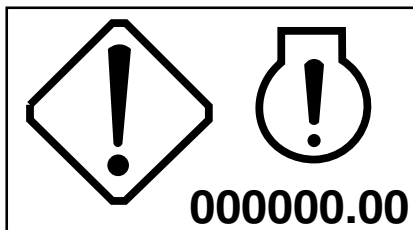
PY46275—UN—07SEP17 Generic Engine Fault - Warn Lamp Status
