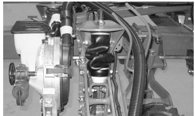
Improperly Rolled Air Spring (Twin Row Planters)
