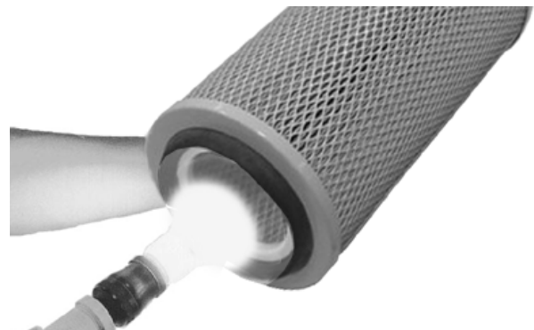
Inspecting filter insert
