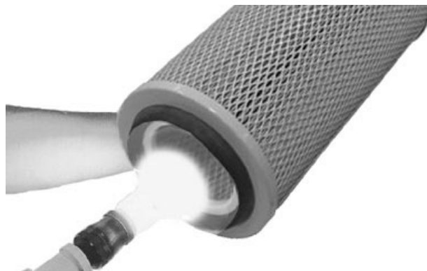
Inspecting filter insert
