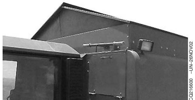
Grain tank extension - harvesting position
