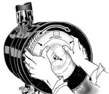
Installing filter insert
