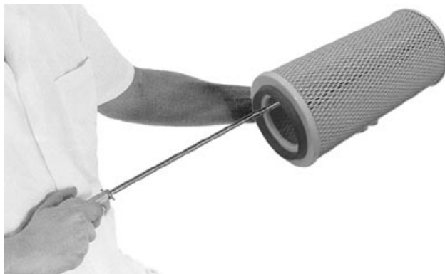
Cleaning the filtering element
