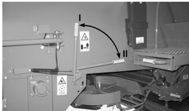
Deflector sheet lever (CWS/WTs)
