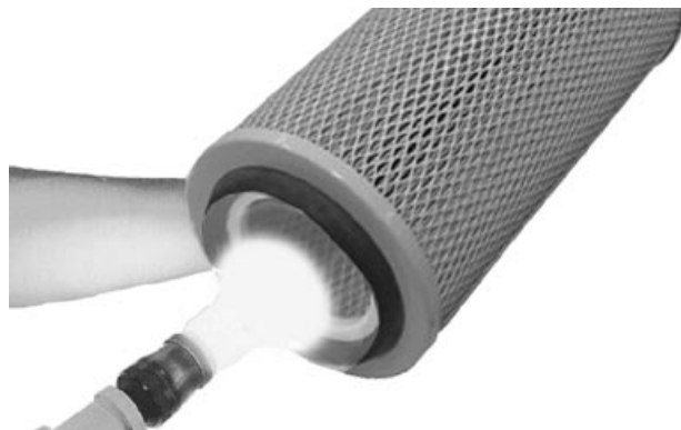
Inspecting filter insert
