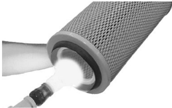
Inspecting filter insert
