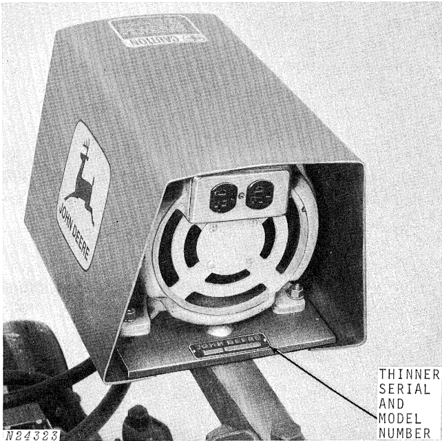
The thinner serial and model numbers are on a plate located on the alternator shield.
