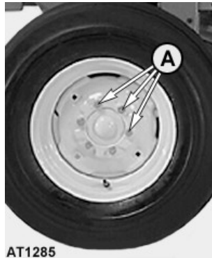
A—Schlüssel an Achsflansch
