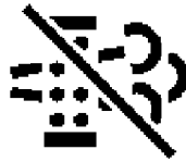
ICONCC059—UN—06JUN13 Automatic Exhaust Filter Cleaning not Activated
