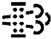
ICONCC058—UN—06JUN13 Automatic Exhaust Filter Cleaning Activated
