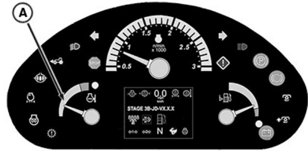
A—Coolant Temperature Gauge
