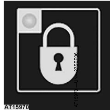
Transport lock switch (with red LED)
