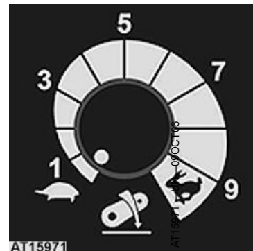
Lowering speed control switch
