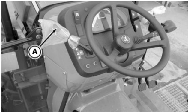
PY34659—UN—13JUL17 Reverse Drive Lever (Mechanically Actuated) (5GL and 5GL-N)
