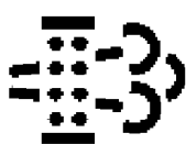
ICONCC058—UN—06JUN13 Automatic Exhaust Filter Cleaning Activated
