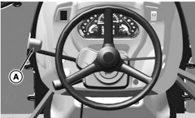
PY31893—UN—26AUG16 Reverse Drive Lever (Mechanically Actuated) (5GV, 5GN, 5GF)
