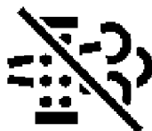
ICONCC059—UN—06JUN13 Automatic Exhaust Filter Cleaning not Activated
