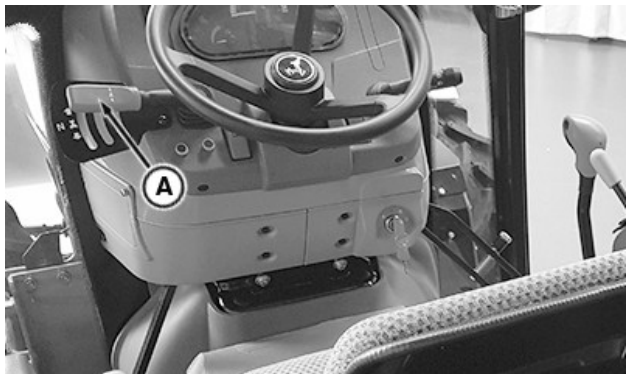
APY11177—UN—14MAY19 Reverse Drive Lever (Electrically Actuated) (5GL and 5GL-N)
