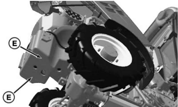
E—Raise Front End of Tractor under the Front Axle Support
