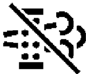
ICONCC059—UN—06JUN13 Automatic Exhaust Filter Cleaning not Activated
