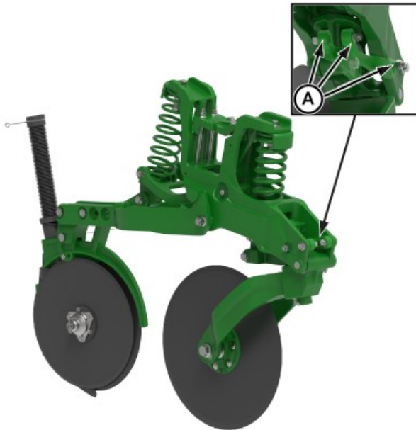
CQ1451982—UN—20MAR26 Cutting Disk Mechanical Spring Linkage Bushing Wear
