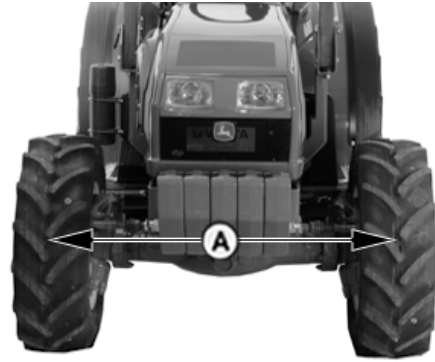
A—Front Axle Toe-In Distance
