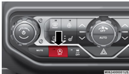
Stop/Start OFF Switch
