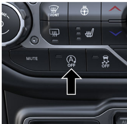
STOP/START Off Switch
