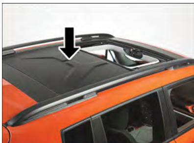
Installing Rear Panel
