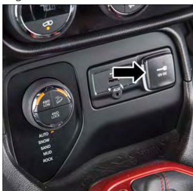
Front Power Outlet
