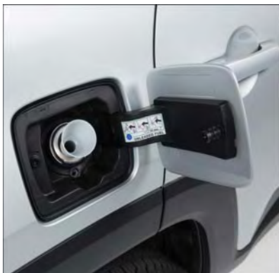
Fueling With Emergency Fuel Fill Funnel
