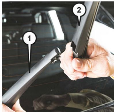
Wiper Blade Removed From Wiper Arm
