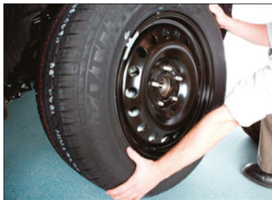
Installing Spare Wheel/Tire
