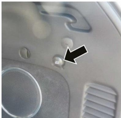
Rear Cargo Power Outlet
