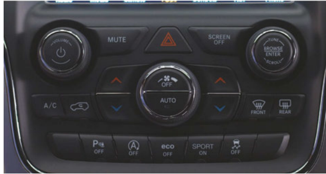
Automatic Climate Controls On The Faceplate
