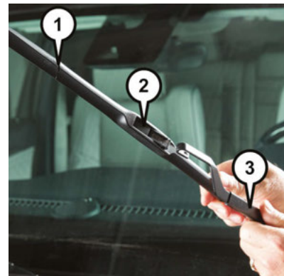
Wiper Blade Removed From Wiper Arm
