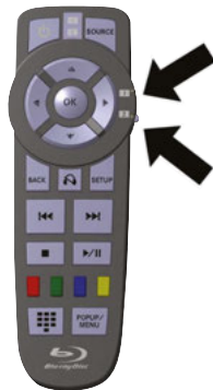
RSE System Remote Control Channel Selectors
