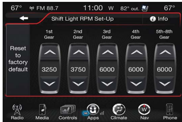
Shift Light RPM Set-Up
