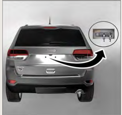
Electronic Release Switch Location
