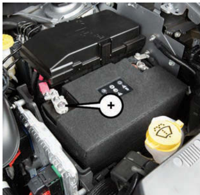
Positive Battery Post
