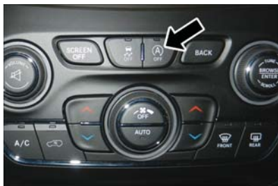
STOP/START OFF Switch
