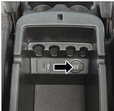
Center Console Power Outlet
