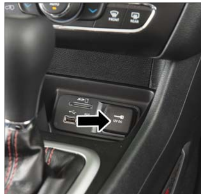
Front Power Outlet
