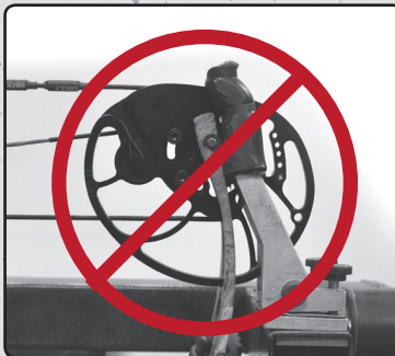
This style of bow press is NOT Hoyt approved for past parallel limb bows and should not be used on those models.
