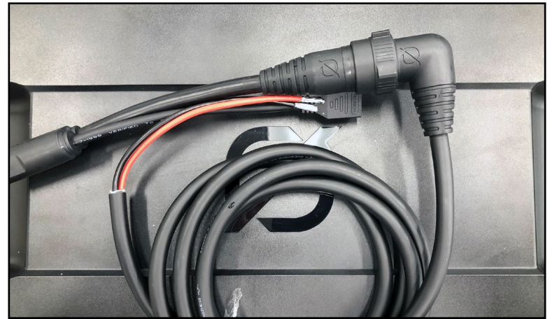
Example of HPP+ Data cable connection point.
