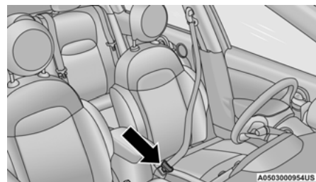
Inserting Latch Plate Into Buckle
