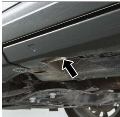
Front Jacking Location
