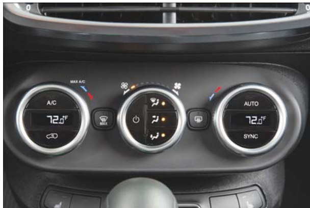
Automatic Temperature Controls (ATC)
