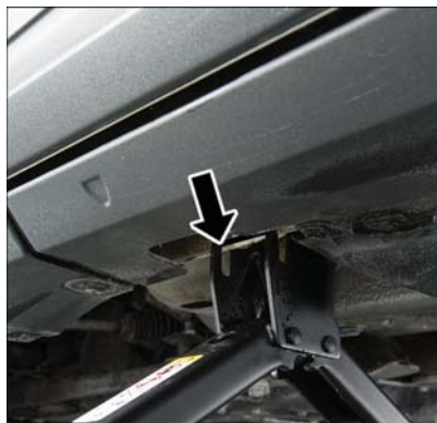
Front Jacking Engagement Point
